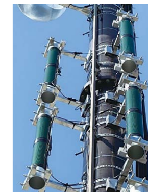
Perovskite solar cell wrapped around a pole
