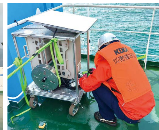
Fixing the Starlink antenna on the ship
